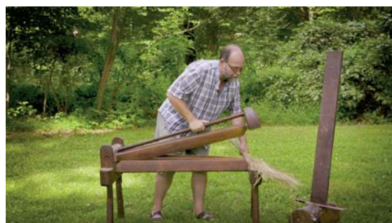
To release the long flax fiber, Tom uses an antique flax brake to crush the woody stalks.
