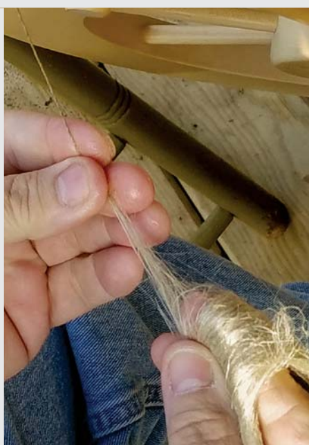
To spin flax from the fold, pull off a length of 5 to 6 inches of flax sliver and fold it over your index finger to spin it easily.
